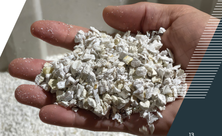
Recycling of agriculture film used in the manufacture of the Holman ECO range
